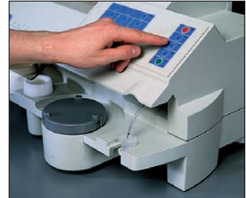
1. Sample is drawn into spiral plater
