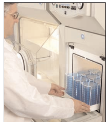
With an airlock, a pull-out tray permits easy transfer of samples from laboratory to workstation
