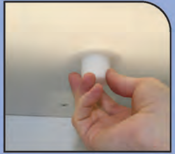
Simple oxygen sensor calibration without removing the sensor from the chamber
