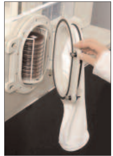
Multi-functional porthole system with latex-free sleeve option
